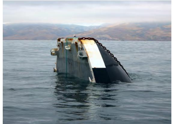
forward cargo and bow rake tanks retained enough air to prevent the barge from "falling over," which left the barge "aground" in a completely vertical orientation.
